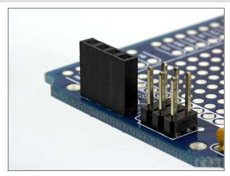
Use the same technique to solder in the 4-pin female header pin (with short pins!) to the location on the bottom of the PCB labeled "BTN1, LED1, LED2, POT1".
